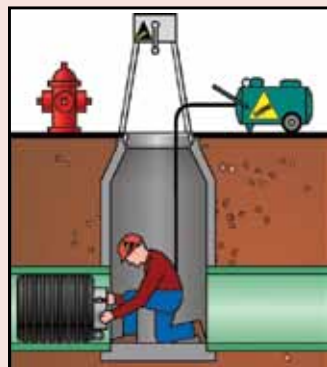
1) Install plug to isolate manhole
