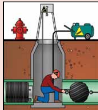
2) Attach Jet-Ball® to tag line and inflate
