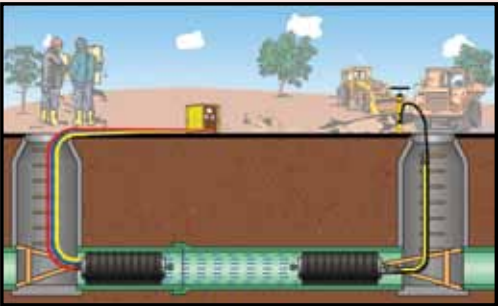
Line Acceptance Test
